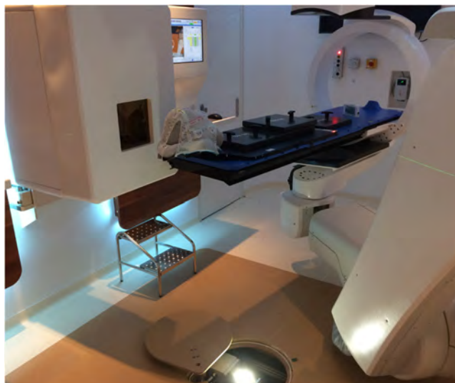
Figure 4. The experimental setup of the Head phantom fixed with the thermo-plastic mask on the BoS frame and loaded with alanine pellets and EBT films. A patient-equivalent weight of 104 kg was placed on the table top and the light based tracking camera including feedback loop to the robotic positioning system corrected for setup errors and the bending of the couch in comparison to the planning CT.
