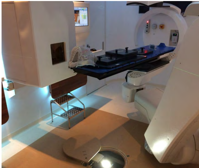
Head phantom – Loaded with alanine
